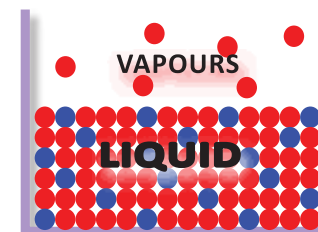
VAPOUR PRESSURE OF A SOLUTION ● particles of a not volatile solute
