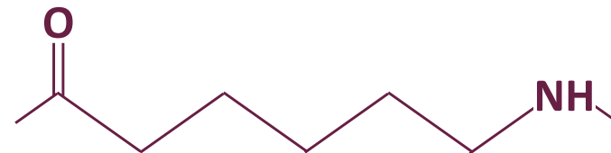
Monomer unit of polycaprolactam (residue of caproic acids \text{H}_2\text{N}-(\text{CH}_2)_5-\text{COOH} )
